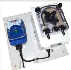
Peristaltic pump controlled by conductivity with electrode's probe Range 240...20.000  $\mu$ S (20 mS) Over feed alarm, settable from 0 to 999 seconds. Pump stops if the probe is dry Automatic priming IP65 Insulation class 2
