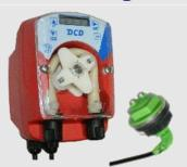
Peristaltic pump controlled by conductivity with electrode's probe Range 240...20.000  $\mu$ S (20 mS) Over feed alarm, settable from 0 to 999 seconds. Pump stops if the probe is dry Automatic priming IP65
