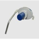
Manual pump, works with the push of a button, dosing adjusted by replacing the end stroke, selectable from 15 cc / 22 cc / 30 cc. It can be installed in any orientation, with aluminium spout. The limit function prevents the over dosage.
